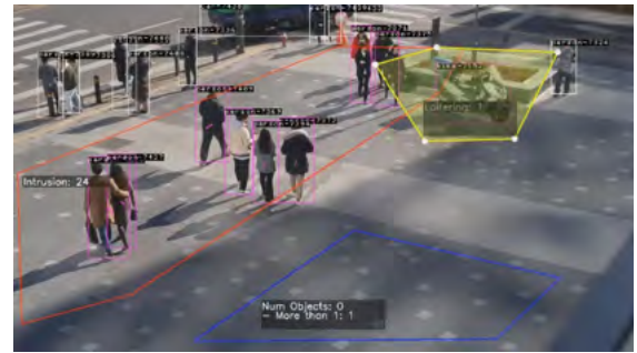
Intrusion, loitering, stop and line crossing
