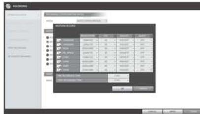
1. Press [MENU] on remote control, and use the direction buttons to select <RECORD SETUP> and press [ENTER]
