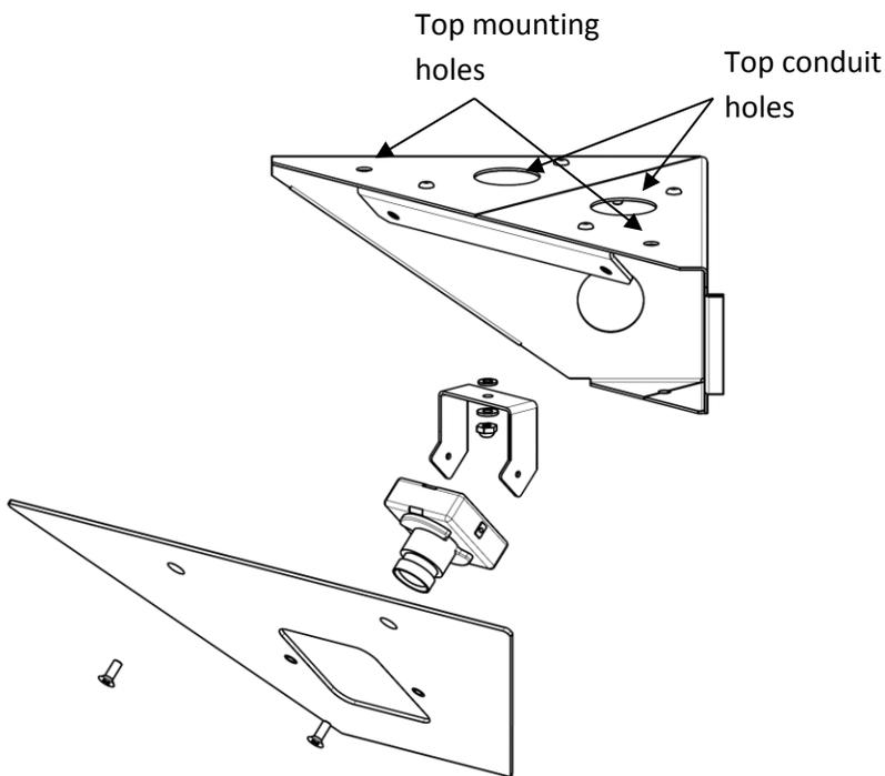
Figure 2 - Exploded View of Corner Camera
